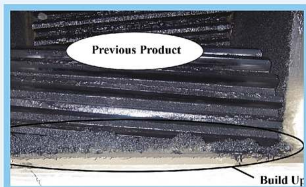
LUBRICANT BUILD-UP EVIDENT
