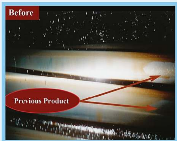
LUBRICANT FILM RUPTURE EVIDENT. LUBRICANT DID NOT MEET OEM RECOMMENDED VISCOSITY FOR OPEN GEARS.
